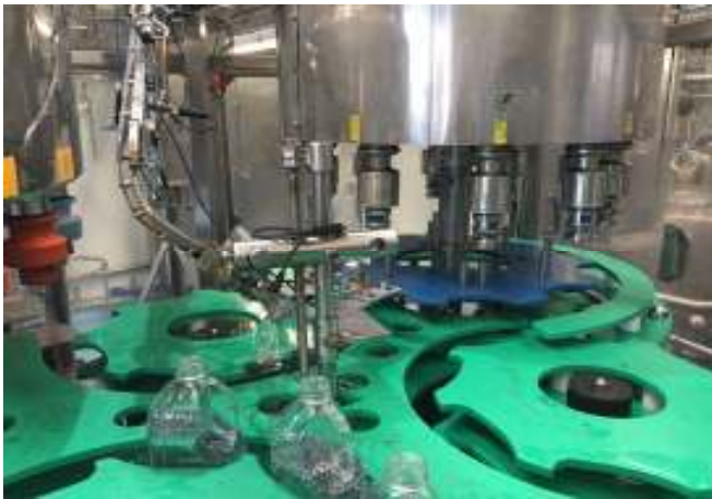
Old capping machine set up with bottle picking off caps from chute
